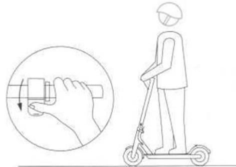
3. now also raise the second foot as soon as the scooter is moving and then press the accelerator lever to accelerate (only accelerate when the speed of the scooter exceeds 5 km/h = kick-start).
