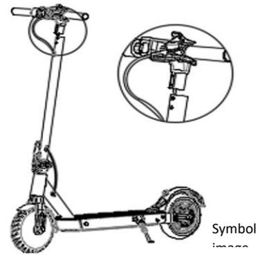
2. mount the handlebar grip on the handlebars
